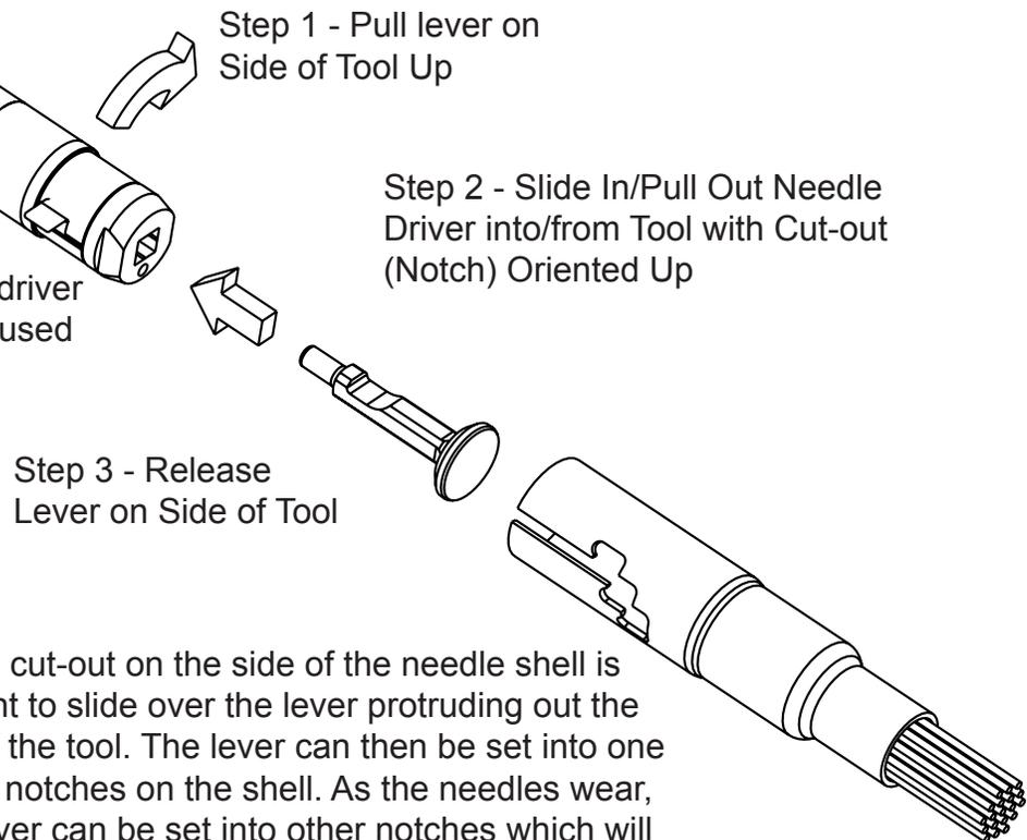
The cut-out on the side of the needle shell is meant to slide over the lever protruding out the side of the tool. The lever can then be set into one of the notches on the shell. As the needles wear, the lever can be set into other notches which will adjust the length of the needles.
